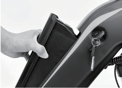
Step 3: The battery can be removed slightly.
