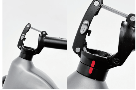
2. Fold the folded seat tube about 90 degrees, rotate the folded seat tube, and align the head tube and seat tube insertion positioning marks.
