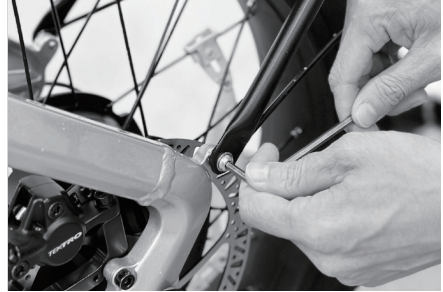
6.Tighten the screws on both sides of the mud-guard.
